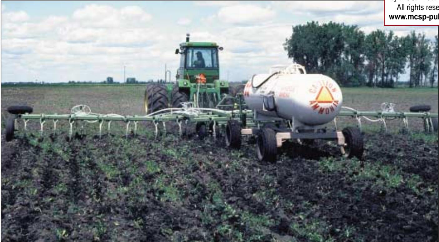
**Figure 6.24.** Anhydrous ammonia has been a popular source of nitrogen for corn since equipment for applying it was developed in the 1940s. Use of modern equipment minimizes the potential for accidents as the operator does not need to transfer the material from a nurse tank to a field applicator tank.
