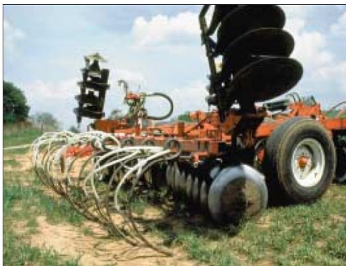
**Figure 6.27.** Application of anhydrous ammonia with a tillage tool saves both time and fuel. This system works well on land which is at the correct moisture for tillage operations.
